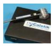
Plastic material manufacturers specify the gas temperature required for welding individual grades of material. Calstik™ is an essential tool for rapidly checking the gas temperature of a hot gas gun.
