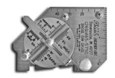
Check Angle of Preparation, Excess Weld Metal, Depth of Undercut, Depth of Pitting, and more.
