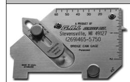
The following measurements are possible in either inches or millimeters: Angle of Preparation, Excess Weld Metal, Depth of Undercut, Depth of Pitting, Weld Throat Size, and more.
