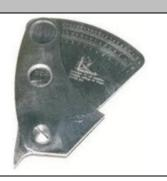
Measuring of fillet weld sizes
