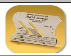
Unequal Leg Measurement Feature used to:
