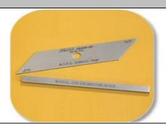
WTPS gauge is precision made from stainless steel. All markings and dimensions are laser engraved for ease and clarity when reading.
